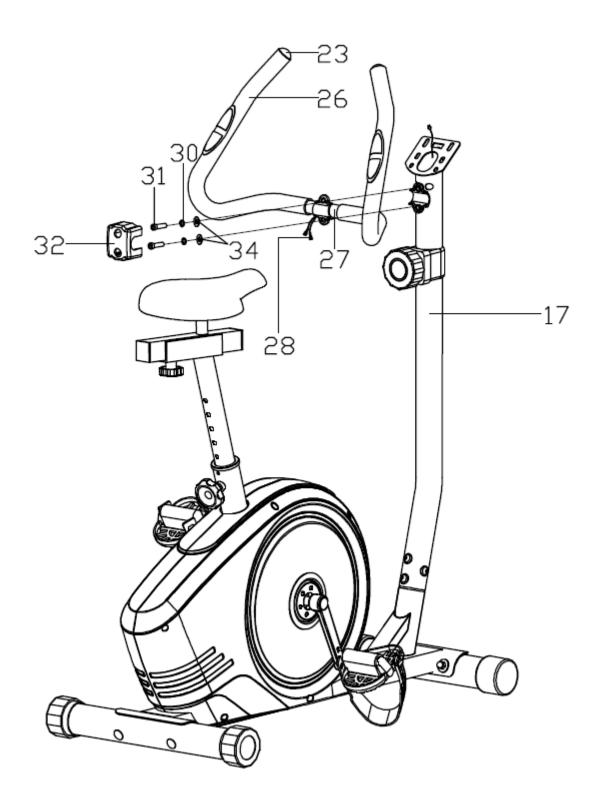
Connect the extension wire(13) and pulse wire(28) to the computer (24), and then install the computer (24) onto the computer bracket on the top of the handlebar post (17) with the cross pan head screw (21) as shown.
