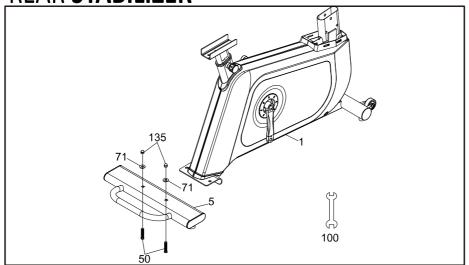
Attach the Rear Stabilizer (5) to the Main Frame (1) by sliding two Cap Nuts (135) two Flat Washers (71) onto two Hex Head Bolts (50), then into the rear stabilizer. Tighten using the 12/14 mm Wrench (100).
