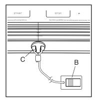
causing the walking belt to slow to a stop. Test the clip by taking a few steps backward; if the key is not pulled from the console, adjust the position of the clip.
