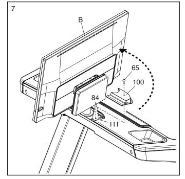
8. Rotate the console assembly (B) to the position shown.
