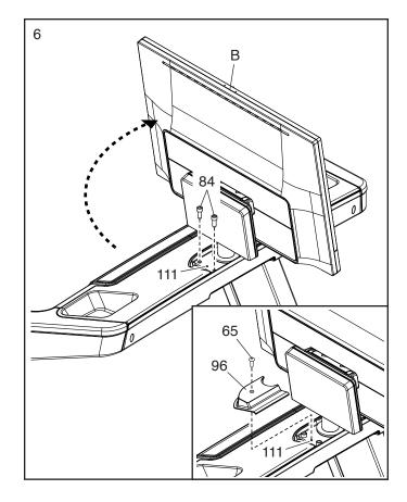
7. Rotate the console assembly (B) back to its original position. Firmly tighten the two 5/16" x 3/4" Screws (84) that you attached in step 5.
