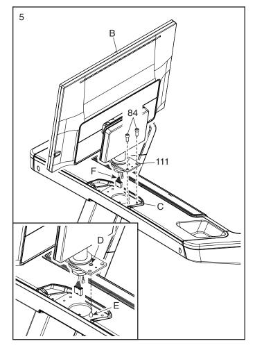
6. Rotate the console assembly (B) so that it faces the opposite direction. Tighten two 5/16" x 3/4" Screws (84) into the Pivot Plate (111); start both Screws, and then firmly tighten them.
