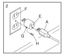
The lug (G) or wire extending from the adapter must be connected with a metal screw (H) to a permanent ground such as a properly grounded outlet box cover. Some 2-pole receptacle outlet box covers are not grounded. Before using an adapter, contact a qualified electrician to determine whether the outlet box cover is grounded. The temporary adapter should be used only until a properly grounded outlet can be installed by a qualified electrician.
