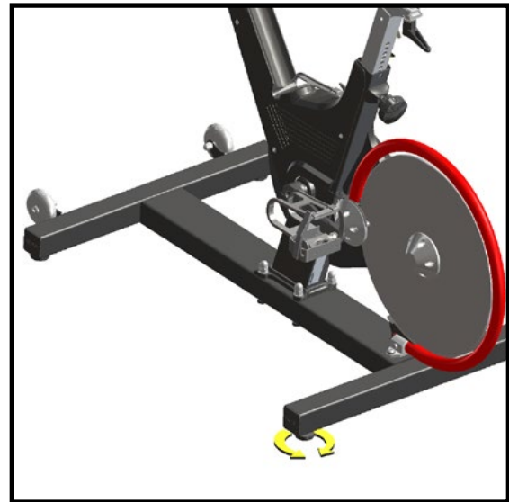
Figure 25. Leveler Foot Adjustment
