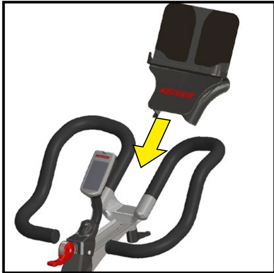
Figure 19. Assemble the device holder to the handlebar
